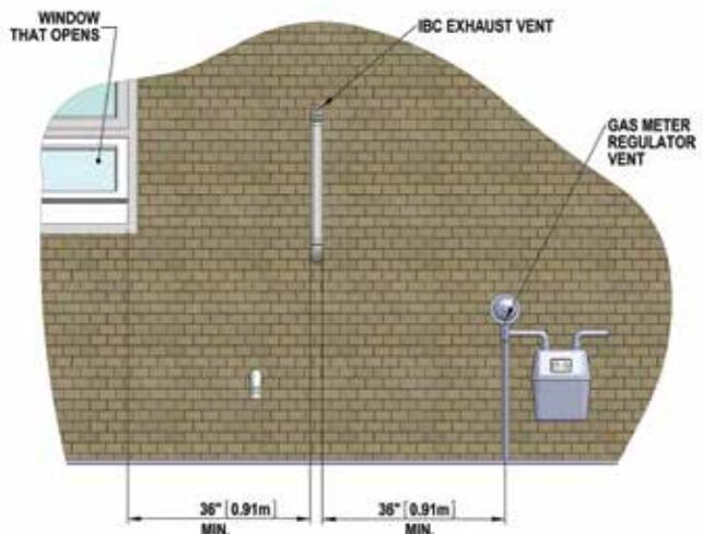
Figure 11: Vent terminal clearances
