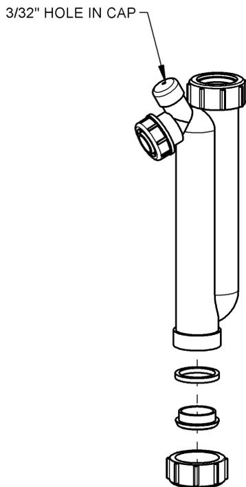
Figure 17: Condensate trap disassembly for cleaning
