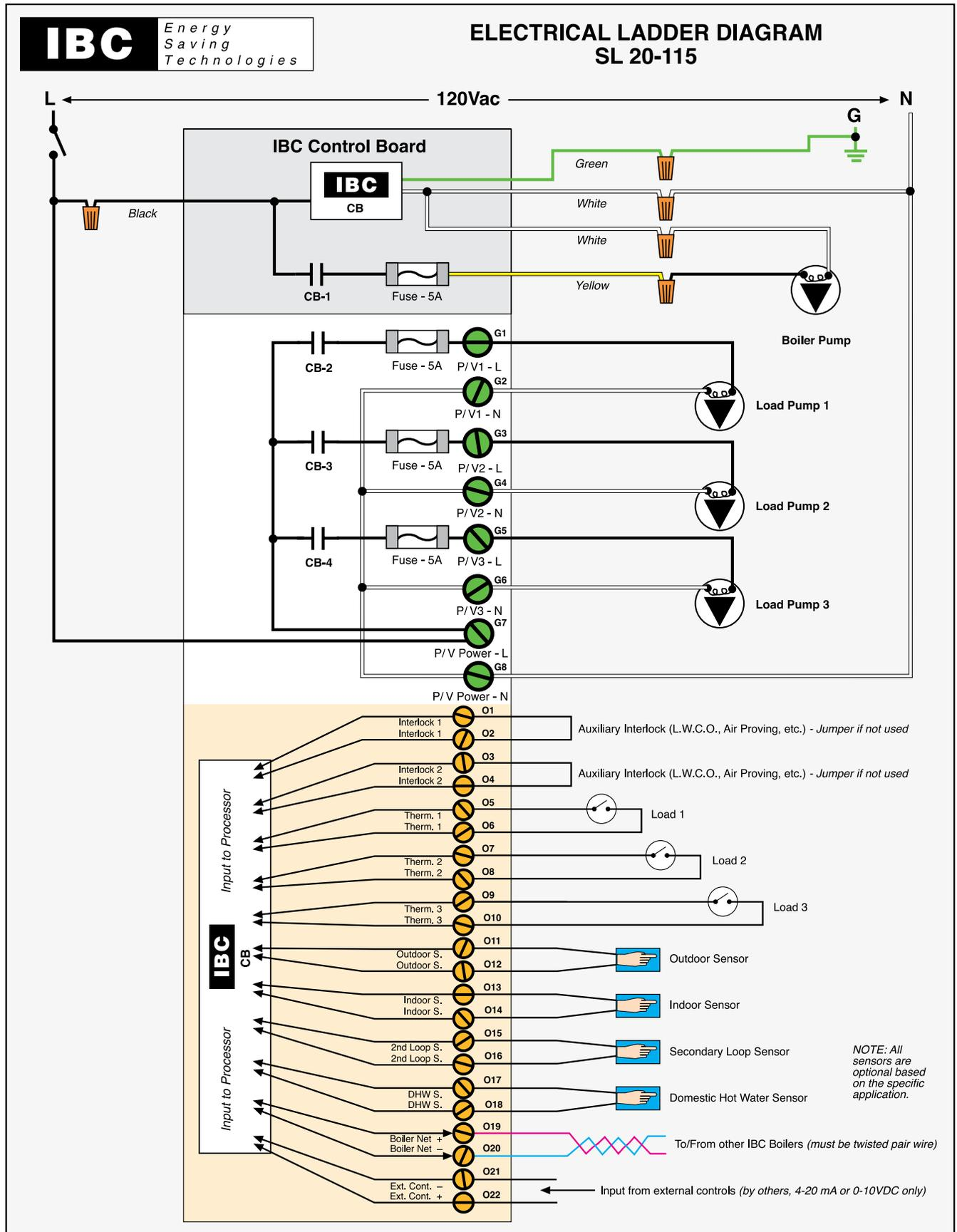
Diagram 6.2-2: Ladder wiring diagram
