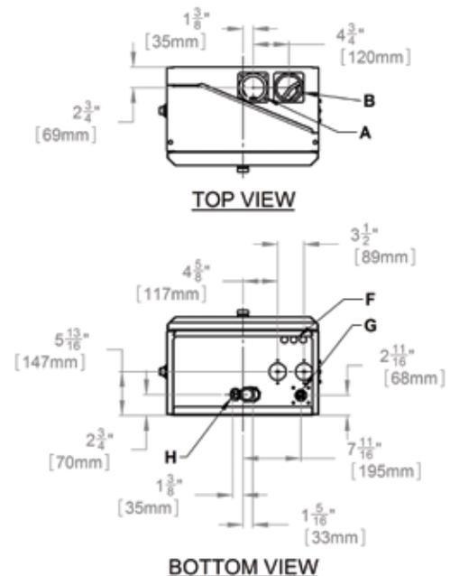
Figure 1a: Dimensions / Connections for SL 20-115
