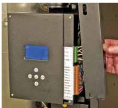
Removing circuit board terminal cover
