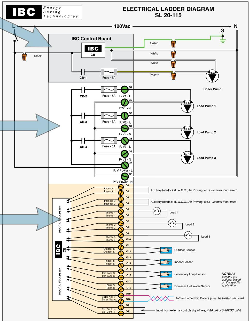
Figure 36: Electrical Wiring Connections (full page ladder diagram at back of this manual)
