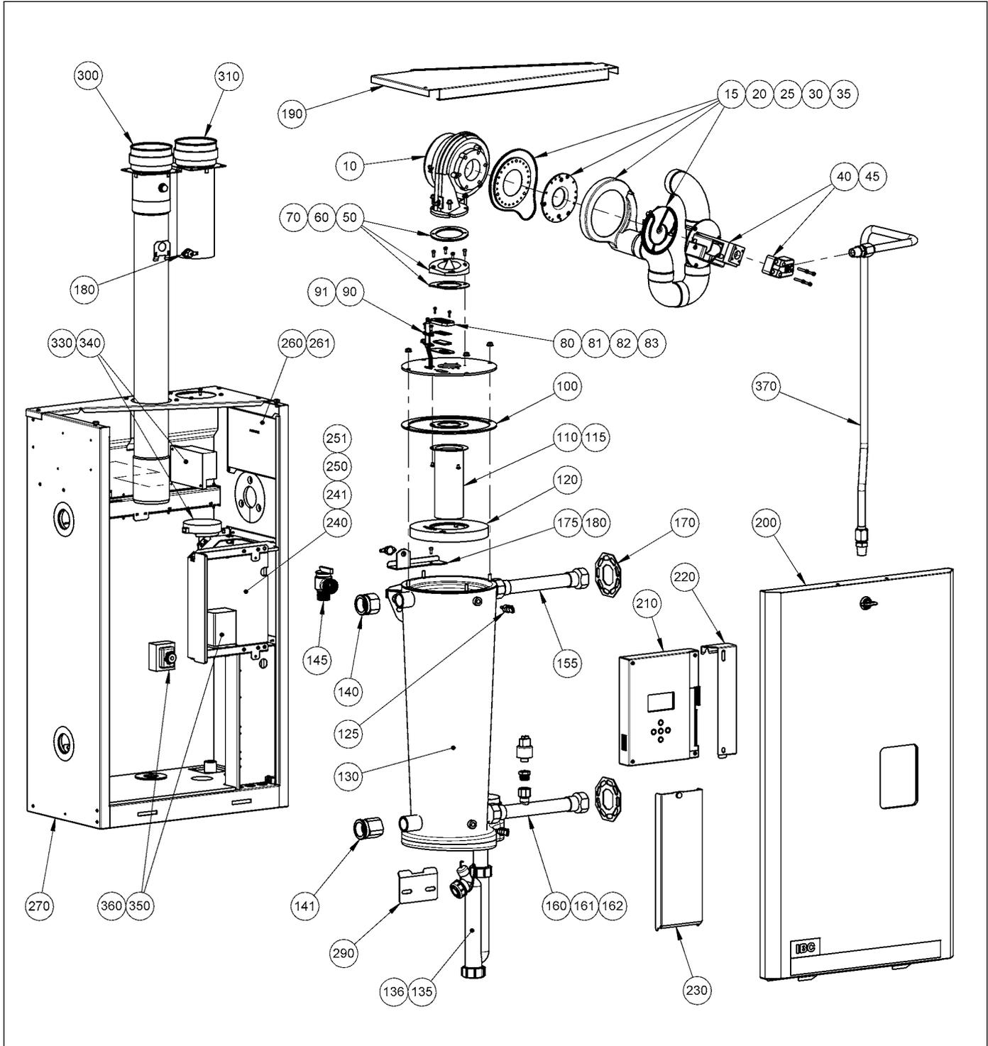
Diagram 6.1-1: Boiler assembly parts
