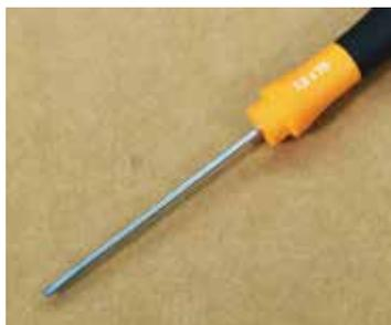
A 2.5 mm Slot screwdriver is required for the bottom terminal strip. Broader or narrower blades may damage the terminal screws.
