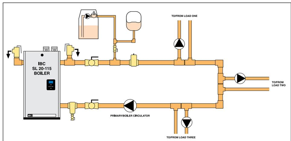
*Figure 24: Basic Primary/Secondary piping with closely-spaced tees concept*
