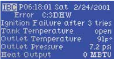
With software versions 3.10.0 and higher, the boiler offers an error status signal feature. *Please see IBC Technical Note: Boiler Status – Analog Output.*
