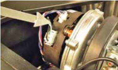
Fan motor electrical connectors
