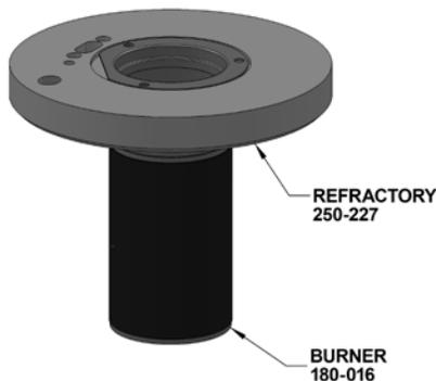
Diagram 6.1-4: Propane Burner Kit, IBC Part #P-103A
