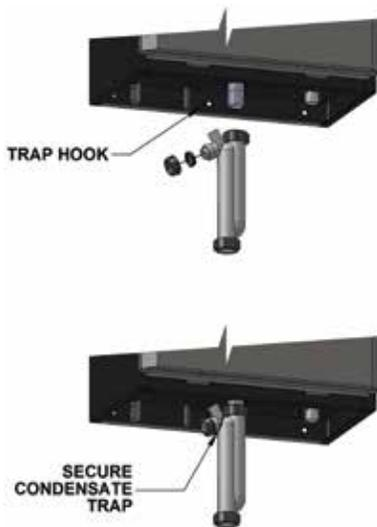
Figure 16: Condensate trap installation
