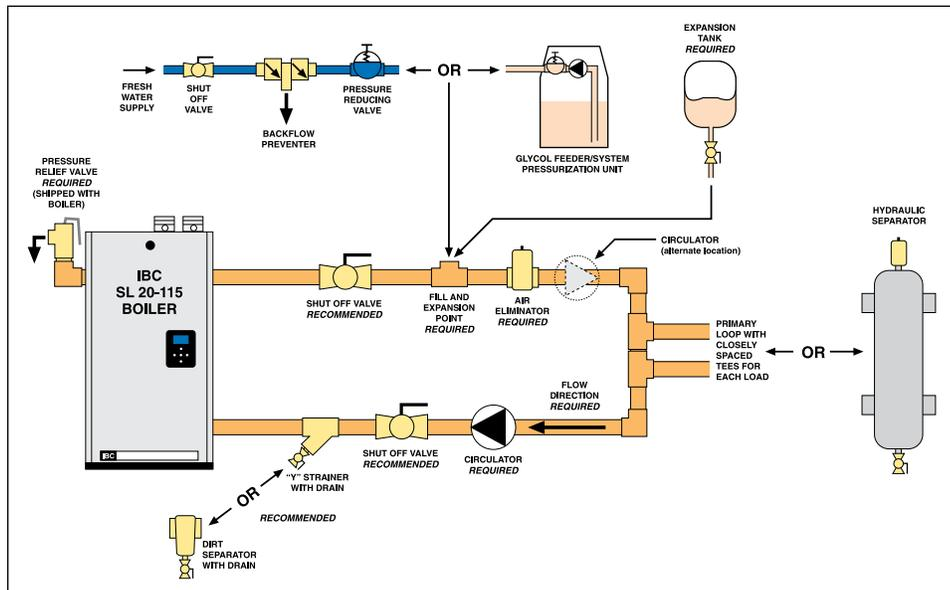
Figure 23: Boiler trim basic options - side piping
