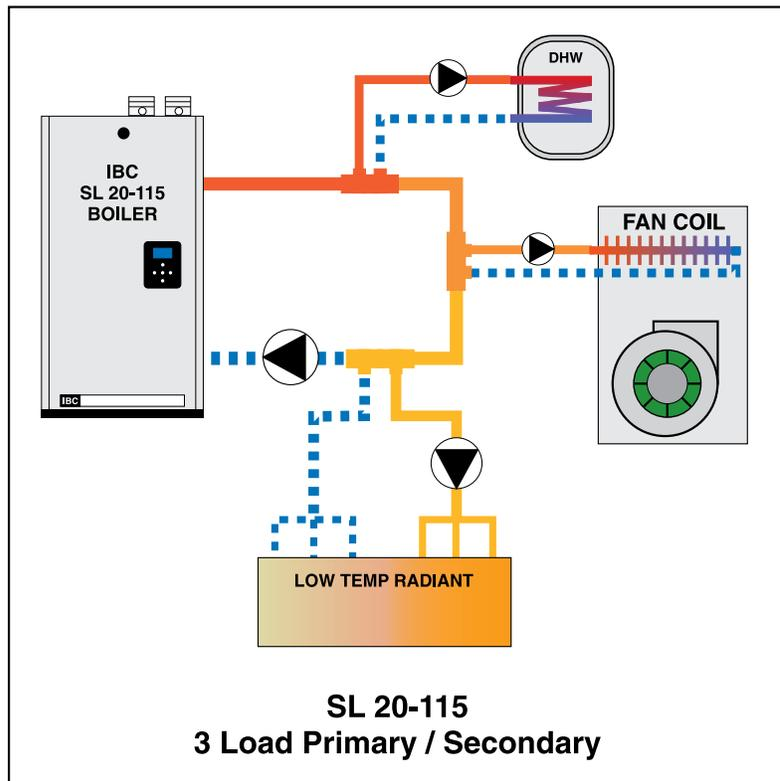
Figure 32: Basic Primary/Secondary, 3 load piping concept
