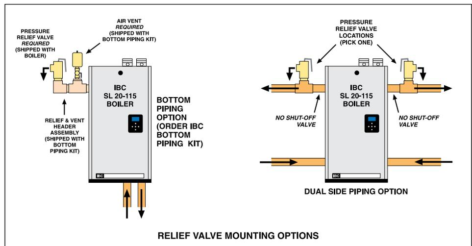
*Figure 22: Relief piping with dual side or bottom piping connections*
