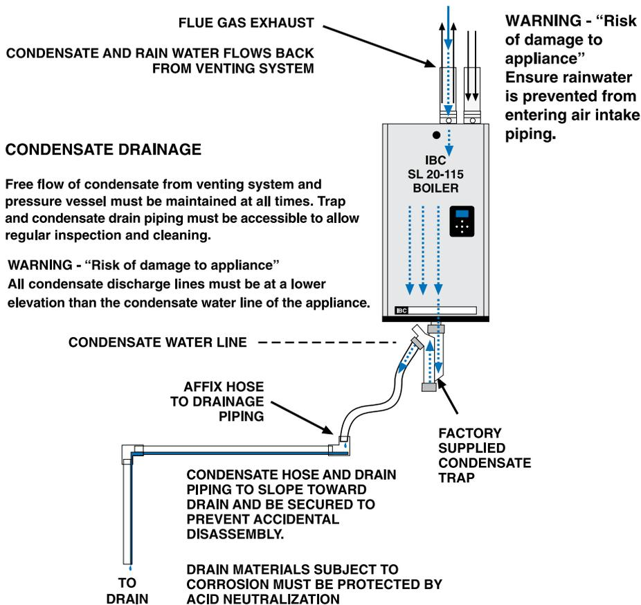
Figure 18: Condensate trap drainage
