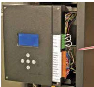
Remove terminal plugs, then circuit board cover
