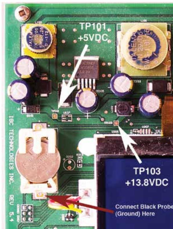
Figure 29 (right): Test points on circuit board for air pressure sensor voltage readings
