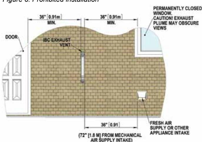
Figure 10: Vent terminal clearances
