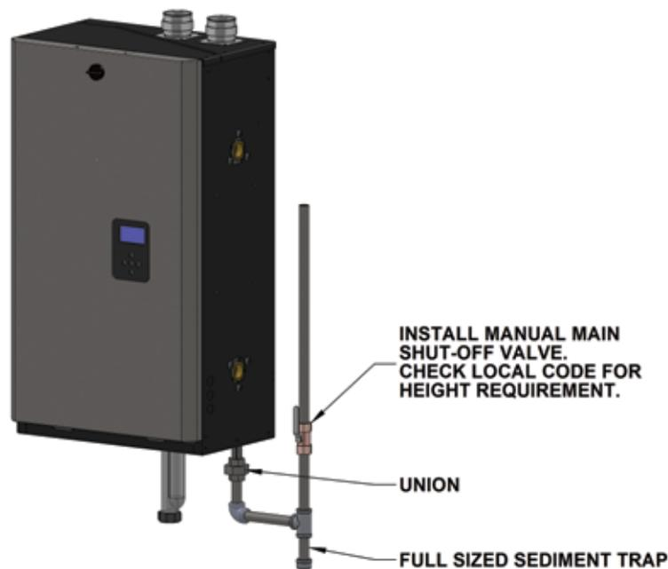
Figure 35: Typical gas piping connection
