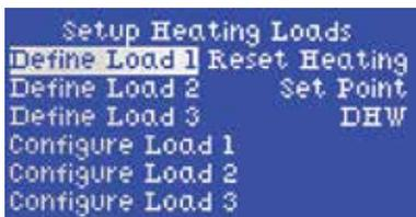
To cause repeated unequal run times (for example, constant 35 vs 5 min. runs) it is necessary to integrate an external load removing relay or timer on one of the heat calls (contact the Factory for details). Do not set each load to the top value, and it is generally better to avoid equal ratings. Note: the priority scale values do not need to add up to 100 – they are relative only to each other.
