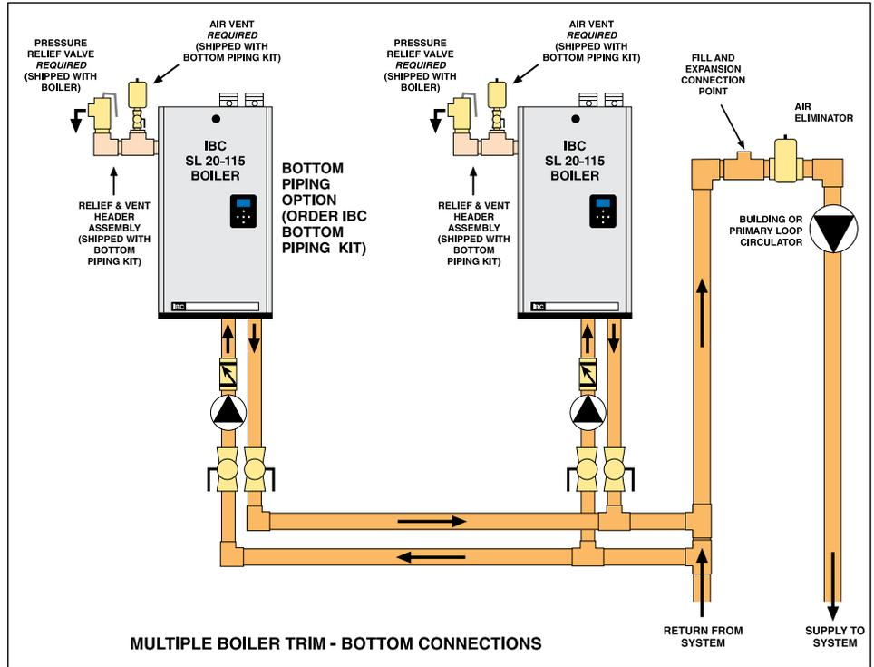
Figure 34: Multiple boiler piping concept
