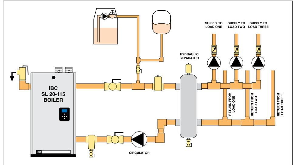
Figure 27: Basic Primary/Secondary piping with hydraulic separator concept
