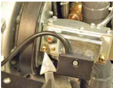
Manifold pressure test port
