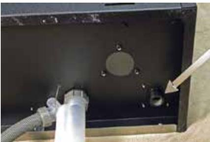
*Gas inlet connection on bottom*
