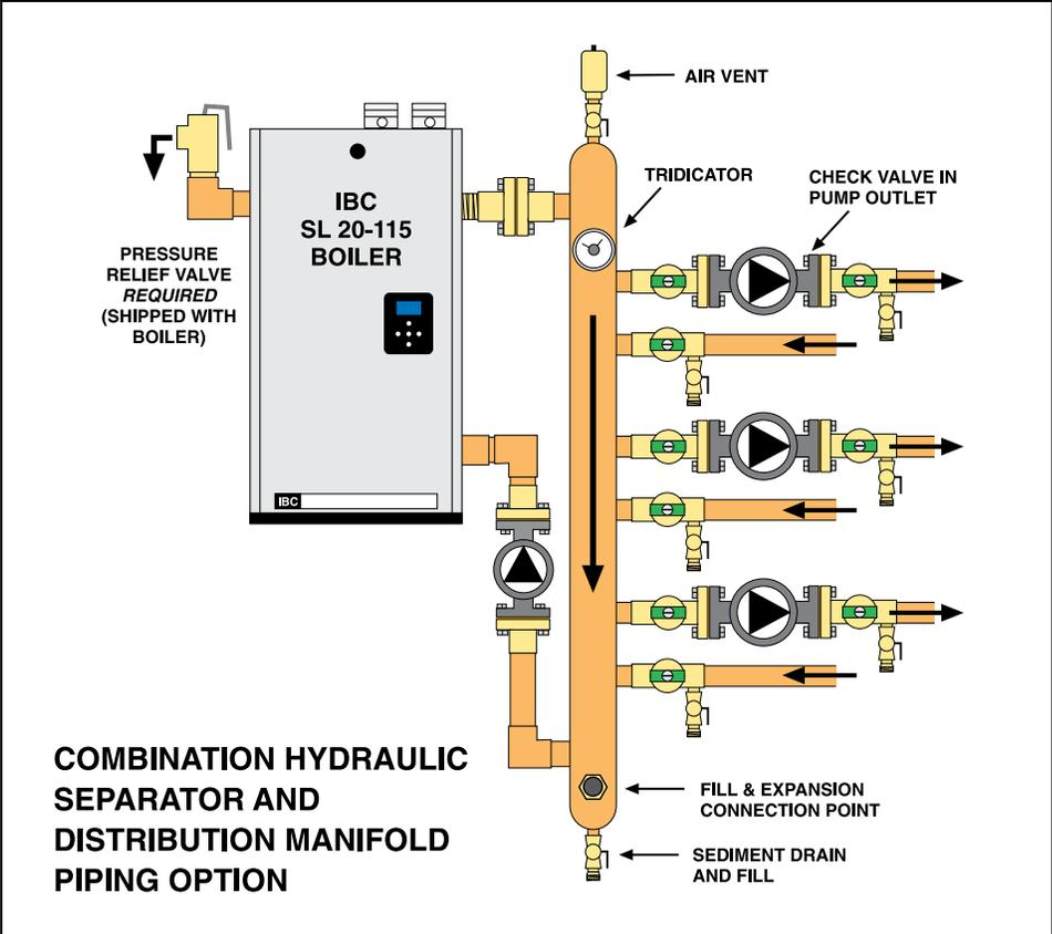
Figure 29: Primary/Secondary piping to a hydraulic separator / distribution manifold
