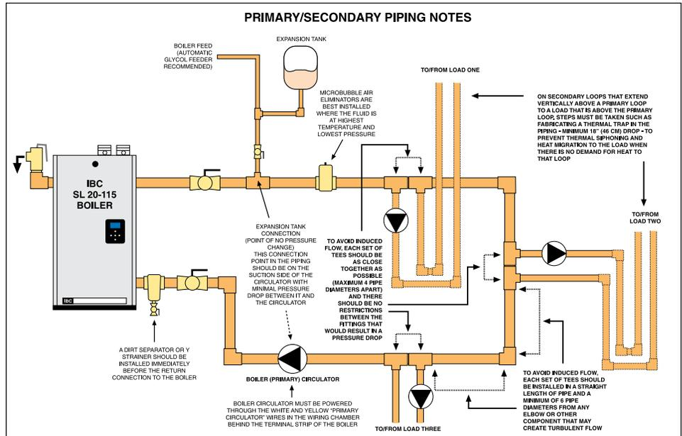
Figure 25: Important Primary/Secondary piping details with closely-spaced tees
