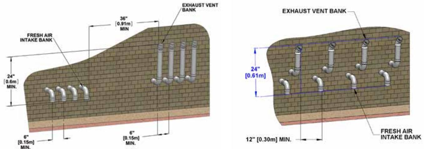
Figure 9: Sidewall vent termination - multiple vent piping configuration
