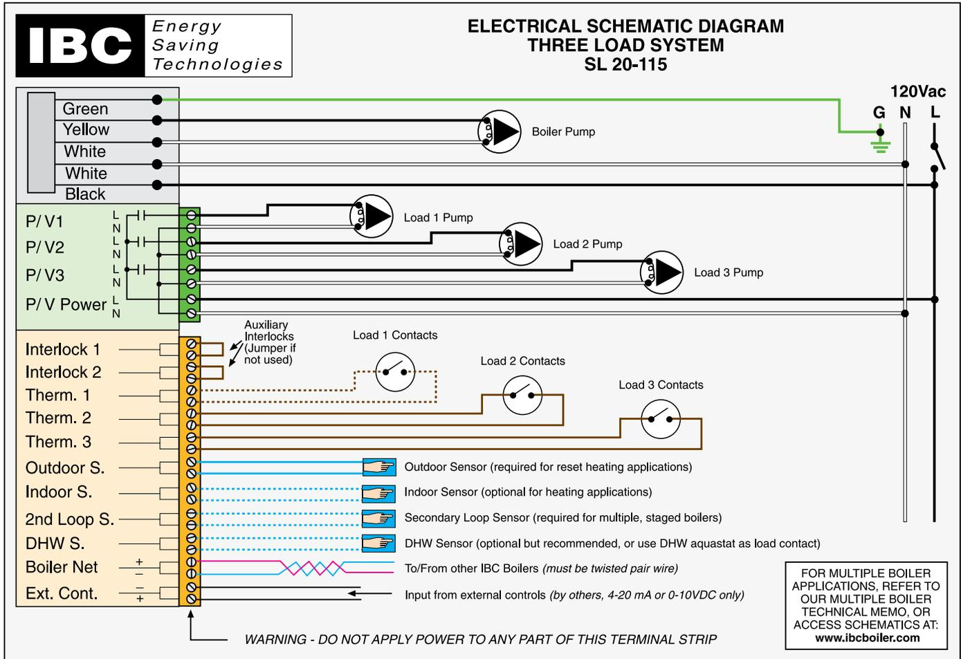
Diagram 6.2-1: Pictorial wiring diagram
