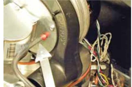
*Fan pressure sensing tube*
