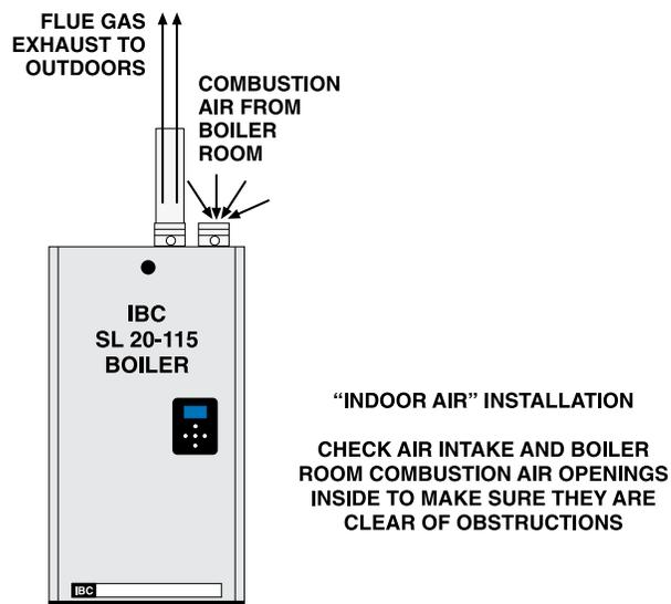
Figure 13: Indoor combustion air intake
