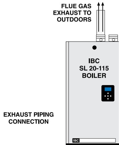
Figure 3: Basic exhaust vent assembly
