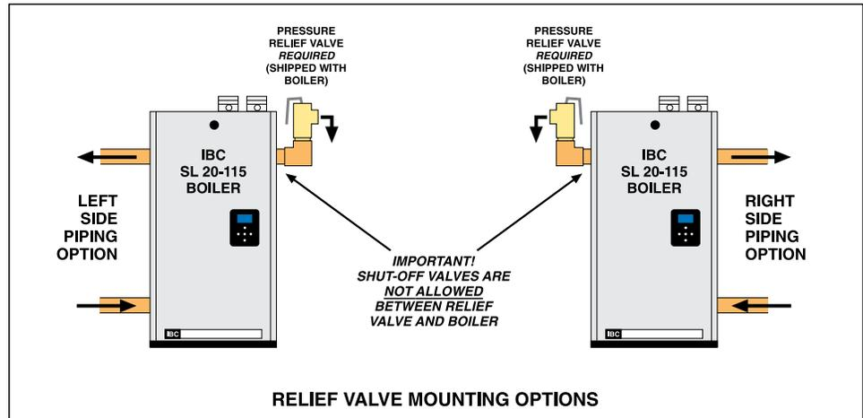
*Figure 21: Relief piping with single side piping connections*
