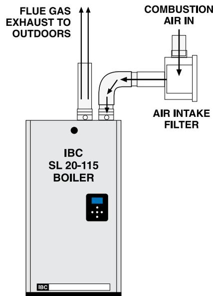
“DIRECT VENT” INSTALLATION WITH INTAKE AIR FILTER
