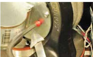
Fan pressure sensing tube
