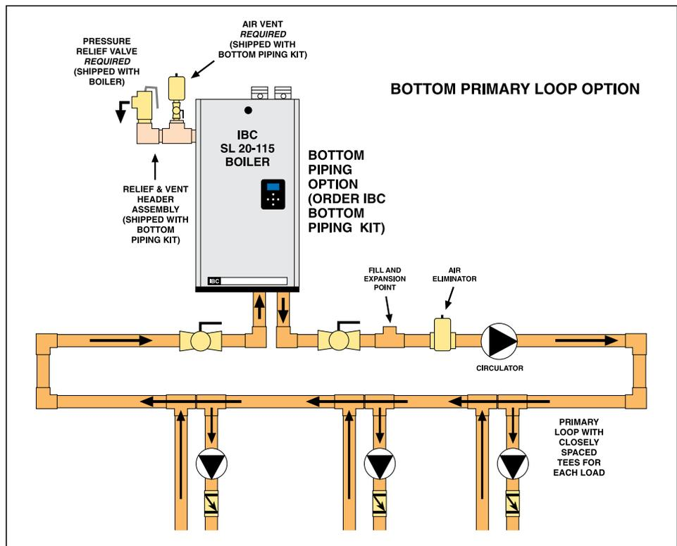
Figure 26: Basic Primary/Secondary piping with bottom piping connection option
