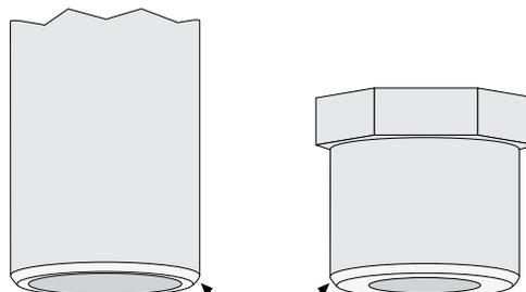
**ENSURE PIPE AND FITTINGS ARE BEVELED FOR TROUBLE-FREE INSERTION THROUGH EXHAUST AND INTAKE PIPE GASKETS**
