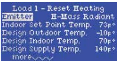
When applied within a condensing boiler, outdoor reset offers direct and significant combustion efficiency benefits by allowing generally lower circulating water temperature. This provides cooler return water to the boiler, promoting more condensation (= energy capture).
