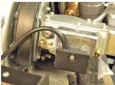
Inlet gas supply pressure test port
