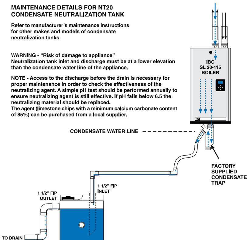
Figure 19: Condensate neutralization tank
