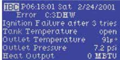
Error displayed after testing ignition safety shut off
