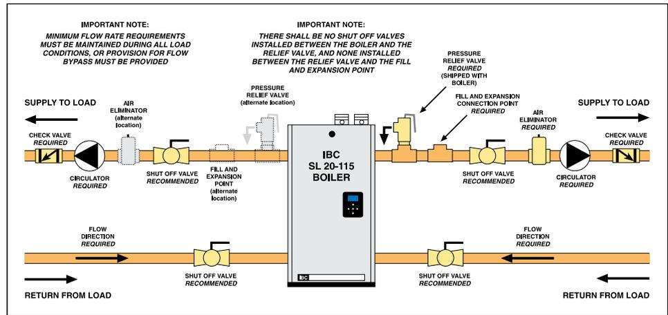
Figure 31: Parallel piping connection to two sides
