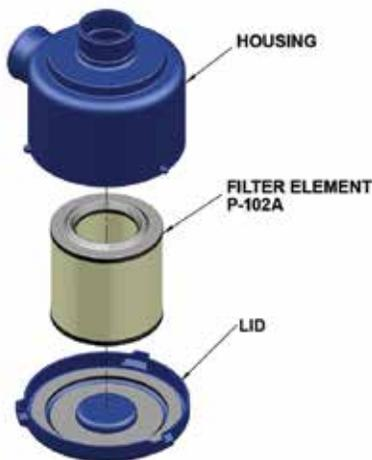
Diagram 15: Intake Air Filter Assembly, IBC Part #SC-100A (Filter Element Alone is IBC Part #P-102A)
