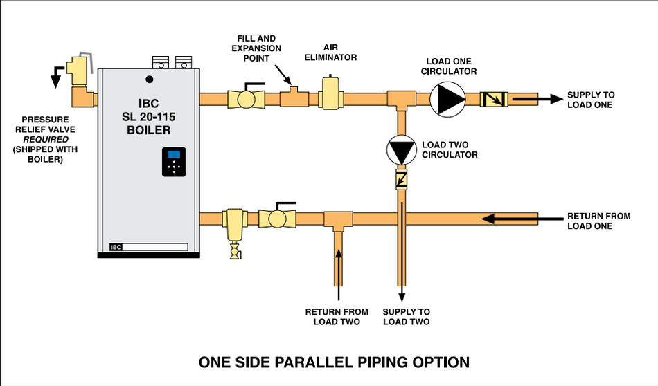
Figure 30: Parallel piping connection to one side
