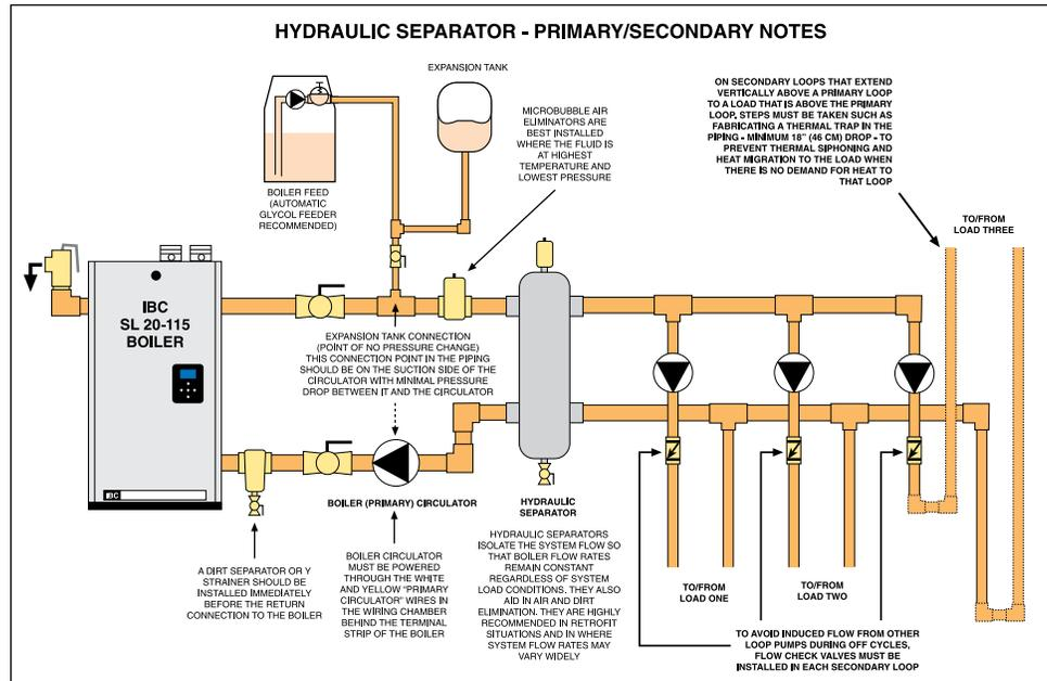
Figure 28: Important Primary/Secondary piping details with hydraulic separator
