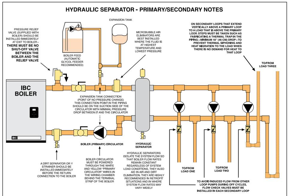
Figure 25: Important Primary/Secondary piping details with hydraulic separator
