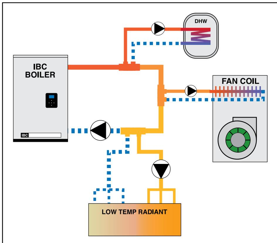
Figure 26: Basic Primary/Secondary, 3 load piping concept
