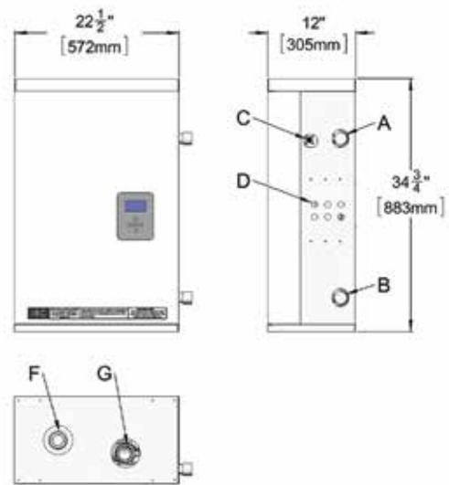
Figure 1b: Dimensions / Connections for VFC 45-225
