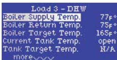
The *Load Status Screen* offers a comprehensive summary of all settings and actual readings for each heating load, eliminating a need to jump between screens while doing an extended watch of boiler operation.
