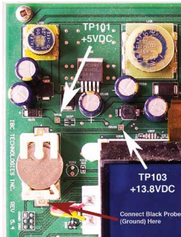
Figure 32 (right): Test points on circuit board for air pressure sensor voltage readings
