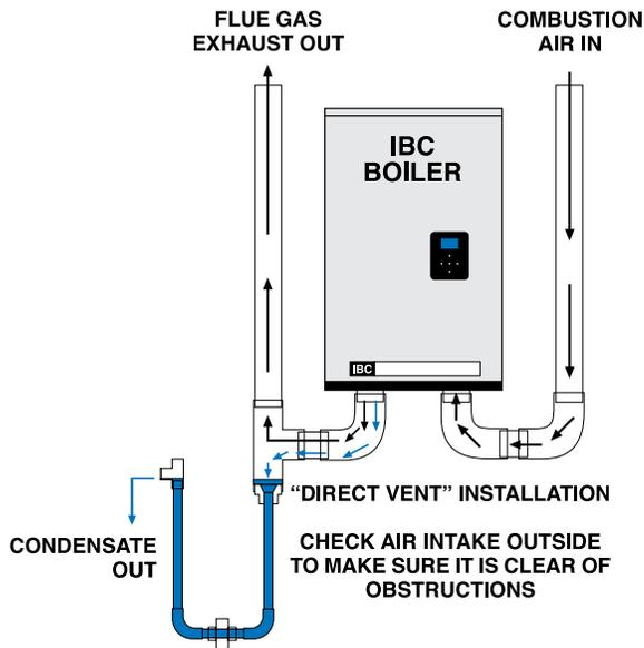
Figure 10: Direct vent - intake, exhaust and condensate removal system
