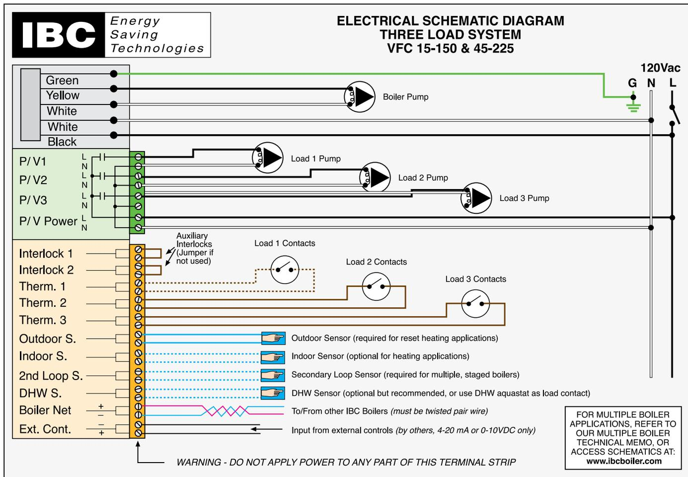
Diagram 6.2-1: Pictorial wiring diagram
