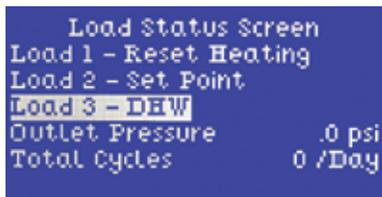
To access the *Main Menu*, touch any key. Move the cursor up or down using the top and bottom keys.
