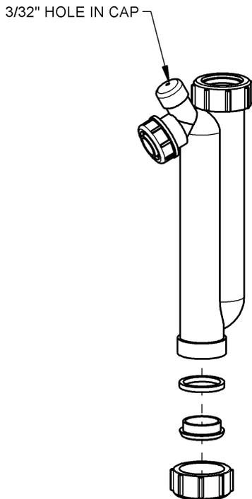
Figure 18: Condensate trap disassembly for cleaning
