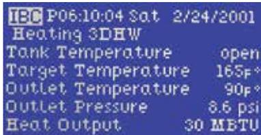
When there is a call for heat from any load, that load is identified at the Status line (e.g. *Heating – RFL (for radiant floor) in place of Standby*). The Target temperature for the relevant load is conspicuously displayed while that load is being handled.
