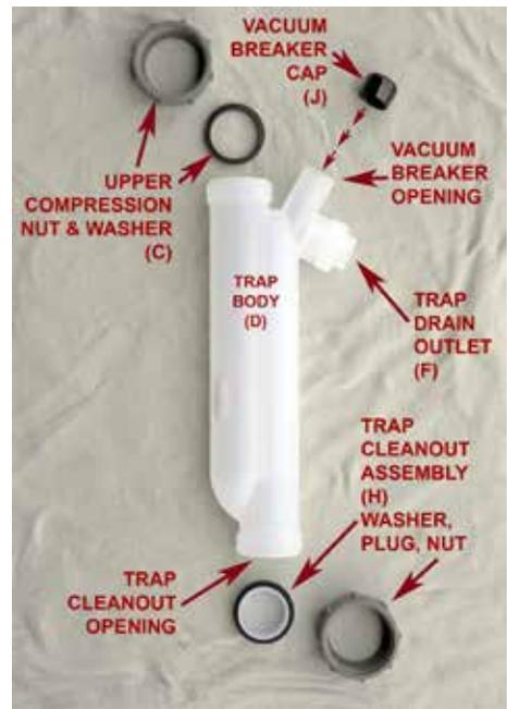
Condensate Trap, disassembled
