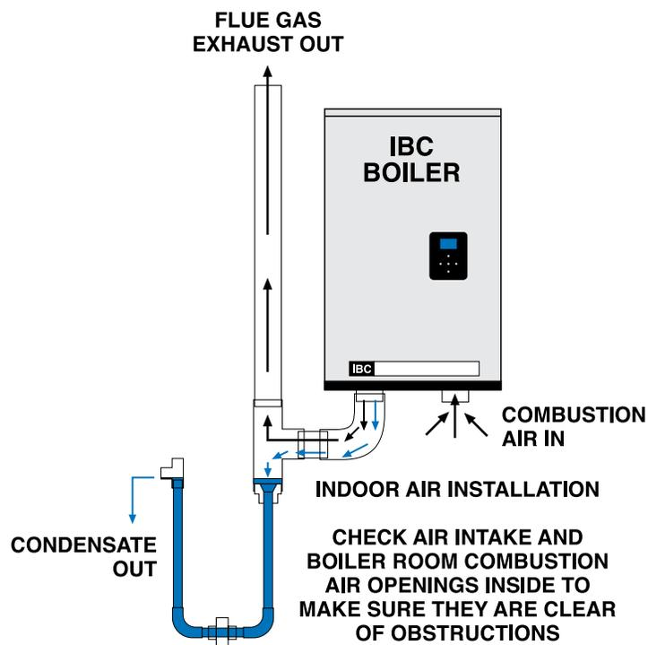
Figure 11: Indoor air - intake, exhaust and condensate removal system
