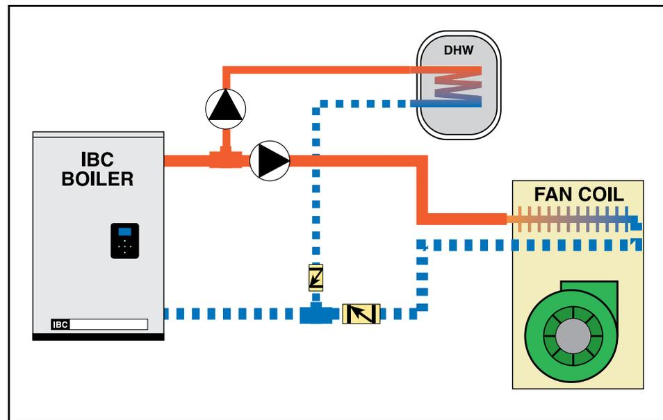
Figure 27: Two pump, two load - parallel piping concept
