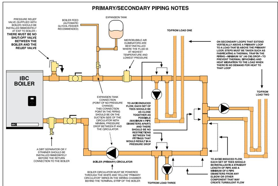
*Figure 23: Important Primary/Secondary piping details*
