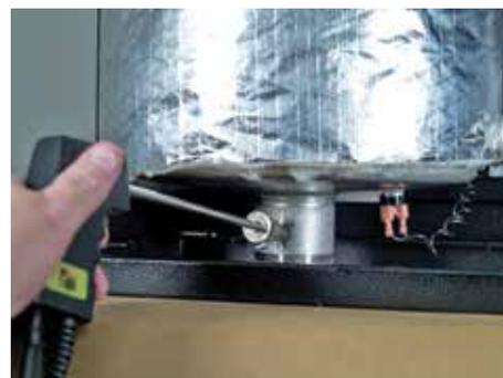
Insertion of flue gas analyzer probe
