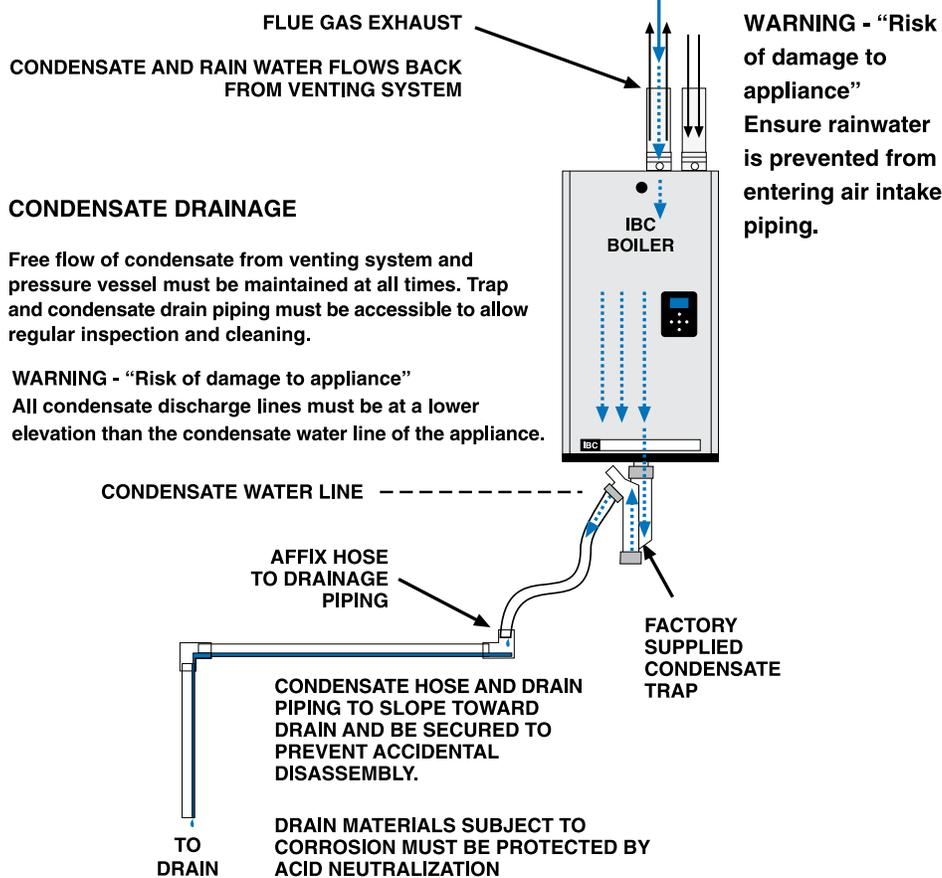
Figure 19: Condensate trap drainage
