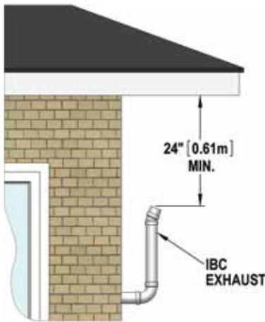
Figure 6: Vent terminal clearances
