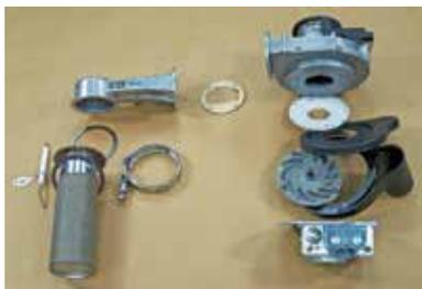
Main combustion components (clockwise from left) Burner, with ignitor and V clamp - Fan coupler - Fan/Blower - Mixing plates & housing - Gas valve
