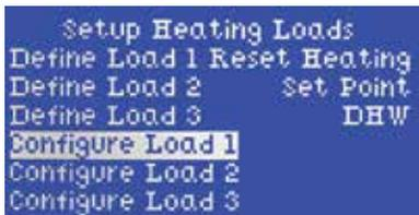
6. Once the appropriate *Loads* are set, use the left-hand key to move back to the *Setup Heating Loads* screen, then move down to *Configure Load 1* (and hit enter).
