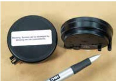
Do not blow into sensor ports
