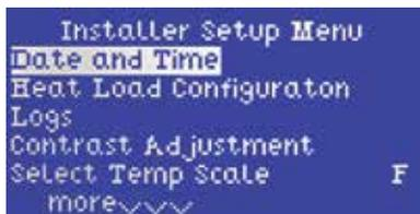
After the boiler is powered up, the installer can use the keypad and display to characterize the application, as follows:
