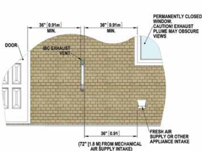
Figure 8: Vent terminal clearances
