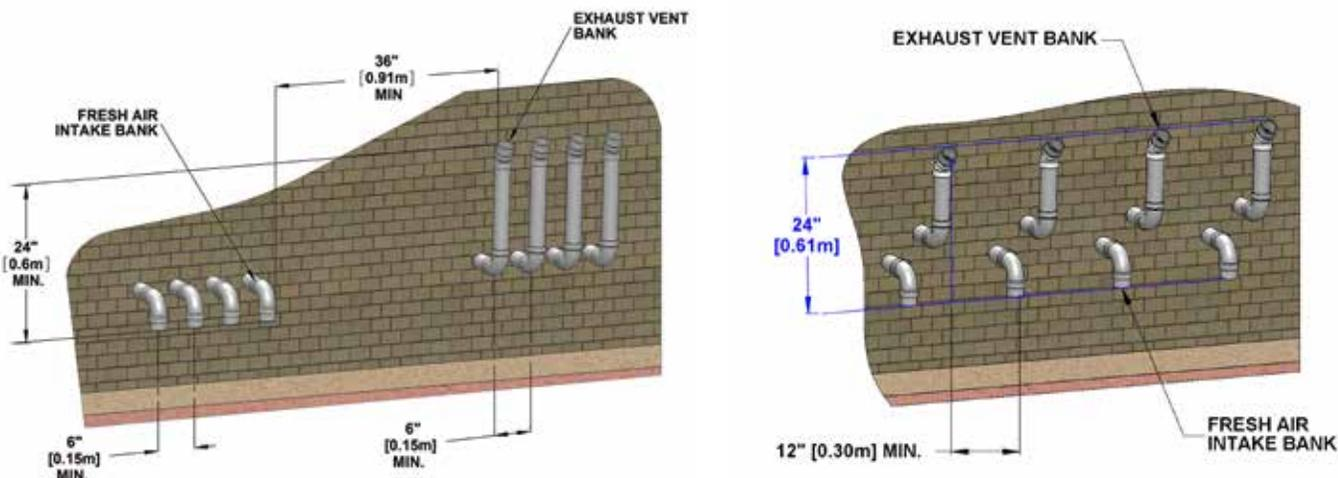
Figure 5: Sidewall vent termination - multiple vent piping configuration
