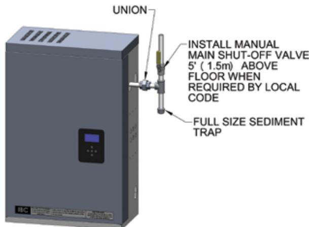
Figure 28: Typical gas piping
