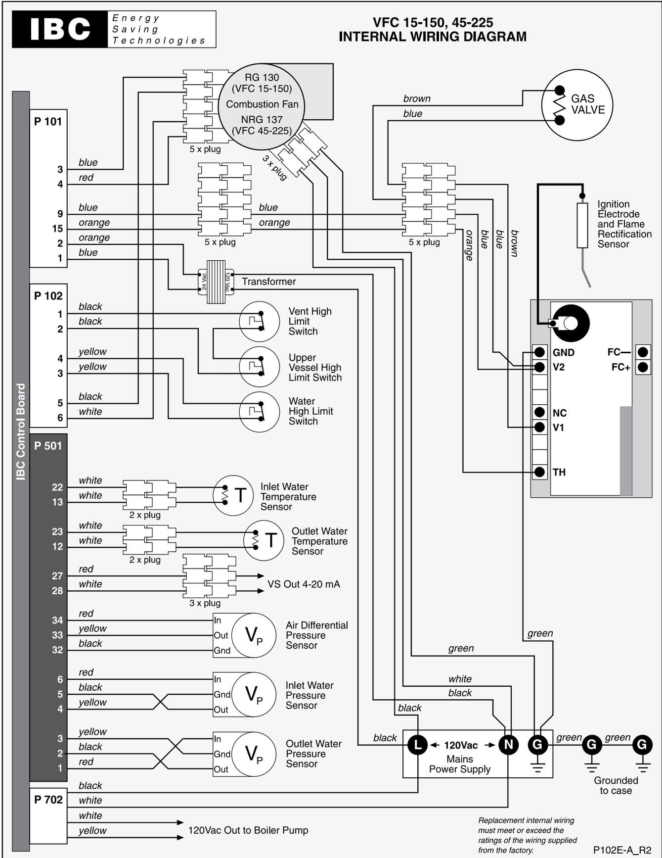
Diagram 6.2-3: Internal wiring diagram
