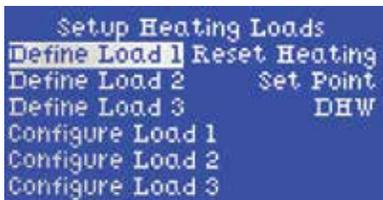
5. Each of the boiler's 3 Load positions can be configured for any type of heating. VFC boilers are factory shipped with default settings as follows: Load 1 set as *Space Heating* or *Reset Heating*, with *High Mass Radiant Floor* set as the terminal type; Load 2 as *Set Point*; and Load 3 as *DHW*. The factory defaults can be changed using the *Define Load 1-2-3* lines to reverse the order, turn off a Load or do whatever the installer desires.
