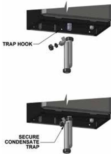
Figure 17: Condensate trap installation
