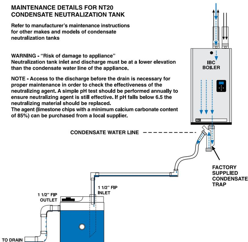
Figure 20: Condensate neutralization tank
