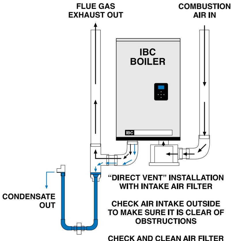
Figure 13: Direct vent - intake, exhaust and condensate removal system with optional air intake filter (filtration may also be used on indoor air applications as required)
