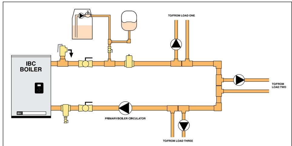
*Figure 22: Basic Primary/Secondary piping concept*
