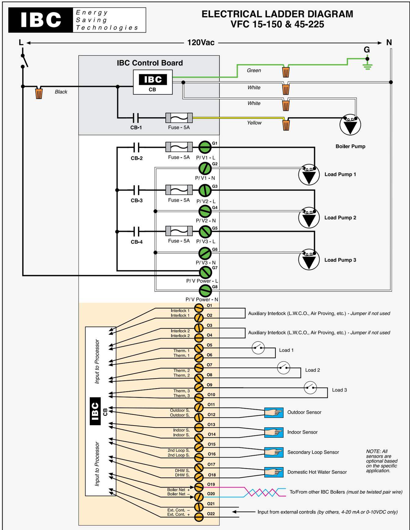
Diagram 6.2-2: Ladder wiring diagram
