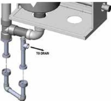
Figure 16: Condensate trap disassembly for cleaning
